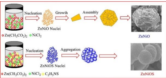
Schematic nucleation mechanism of micro rose-like ZnNiO and nano-sphere ZnNiOS particles
